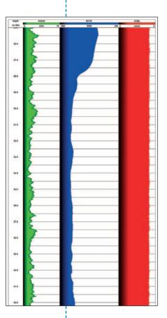
Example of data created by the Impeller Flowmeter probe.
