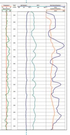
Example of data created by the Electric Log probe.
