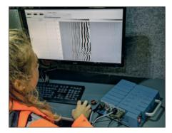
**Winlogger:** MS Windows based operating system for the Micrologger2, provides field acquisition capability. In-house processing, interpretation and reporting is undertaken. *See page 17*
